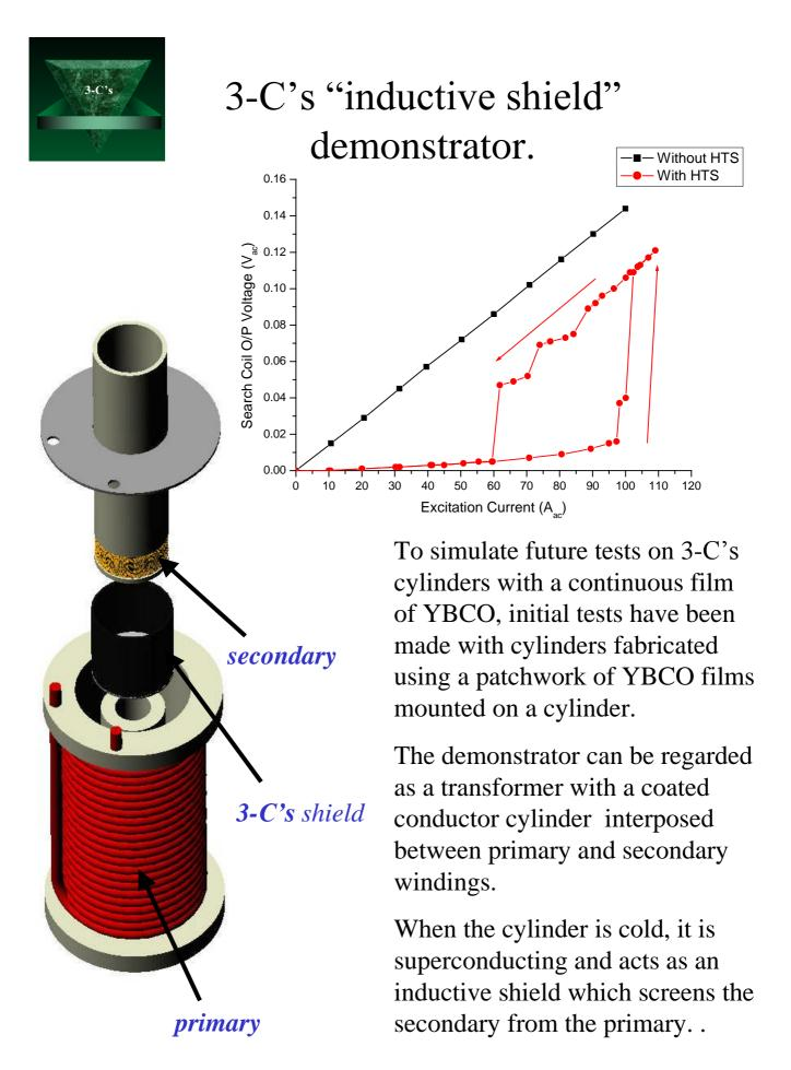
**Potential applications** – FCLs, self-limiting transformers and also shields for low-noise sensors.
