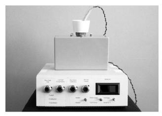
Inspector Hall equipment showing the controller, magnetic sensor unit and sample holder.
