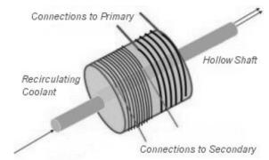
Proposed single layer test structure for a step-up transformer. Similar structures could be used to demonstrate FCL devices (resistive and inductive), SMES modules and a linear motor module
