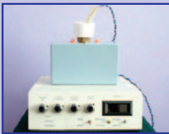
Inspector Hall equipment showing the controller, magnetic sensor unit and sample holder.
