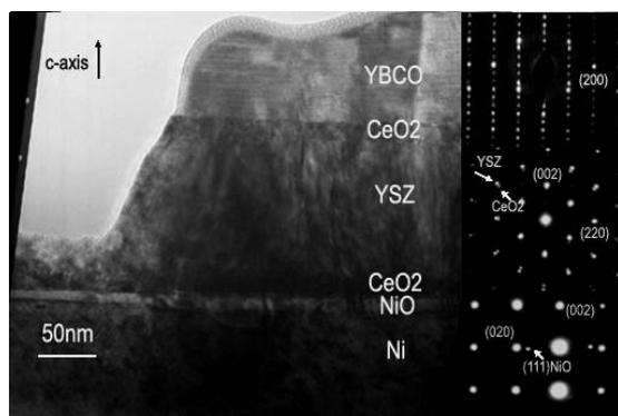
**Figure 7.** TEM image of buffer layer/YBCO structure together with corresponding diffraction patterns confirming transmission of the biaxial texture through the layers.
