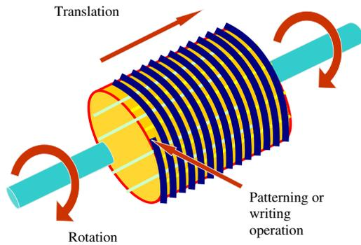
**Figure 1.** Buffer and YBCO layer deposition on an IBAD textured former followed by laser scribing to ‘pattern’ a coil—similar to a screw cutting operation on a lathe. A similar structure could be achieved by an IBAD beam writing process followed by buffer and YBCO layer depositions.
