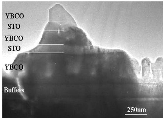
**Figure 6.** TEM image of YBCO triple layer.
