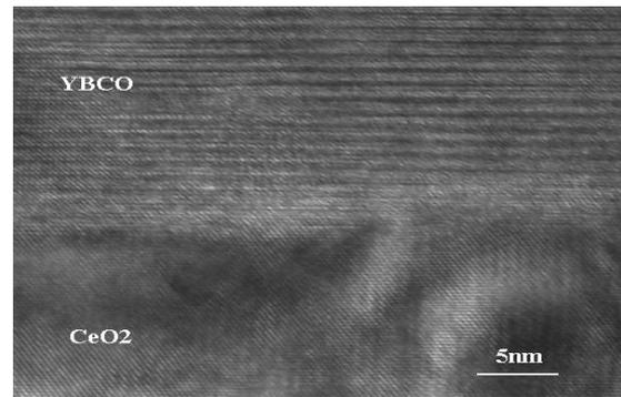
**Figure 8.** High resolution TEM image of YBCO/ $\text{CeO}_2$  interface.
