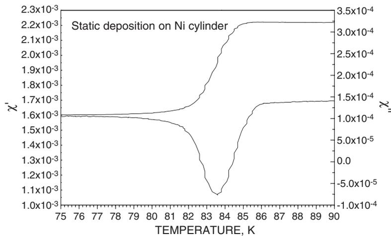
**Figure 4.** AC susceptibility measurement on a single YBCO layer deposited statically on a curved Ni tape.
