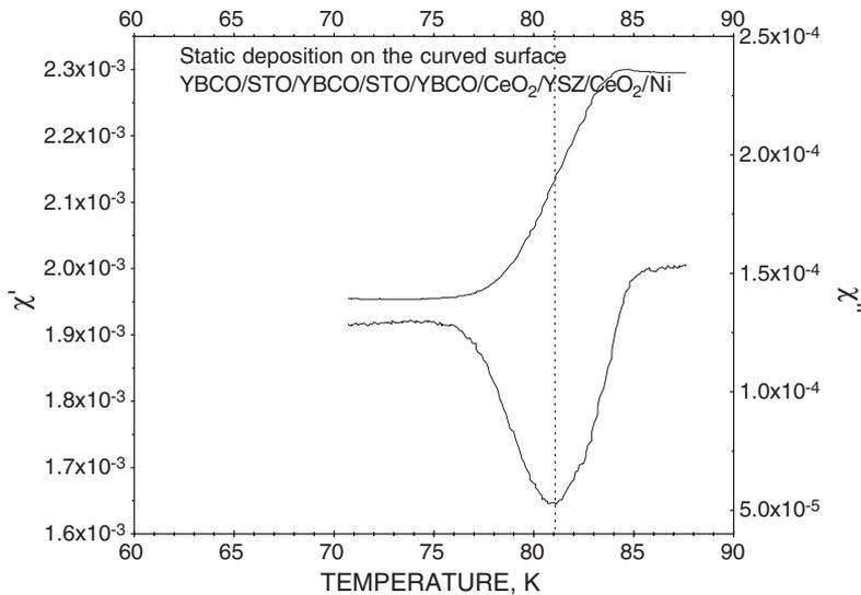
**Figure 5.** AC susceptibility measurement on a triple YBCO layer deposited statically on a curved Ni tape.
