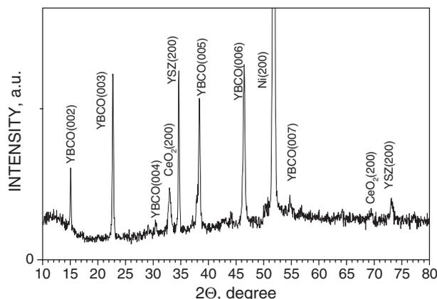
**Figure 3.** XRD scan of single YBCO layer on C/Y/C buffers deposited statically on a curved Ni tape.
