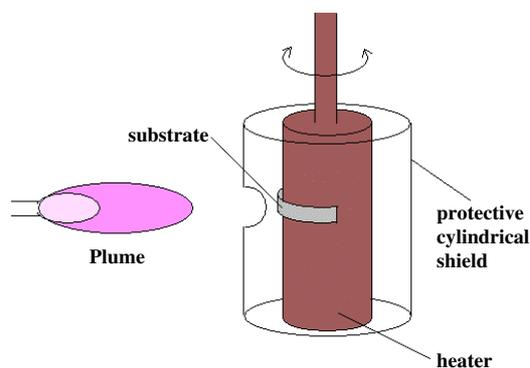
**Figure 2.** Schematic diagram of the rotating cylindrical heater in the PLD chamber.
