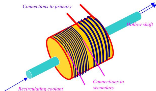
**Figure 9.** Proposed single-layer test structure—for a step-up transformer in this case. Similar structures could be used to demonstrate FCL devices (resistive and inductive), micro-SMES modules and a linear motor module.
